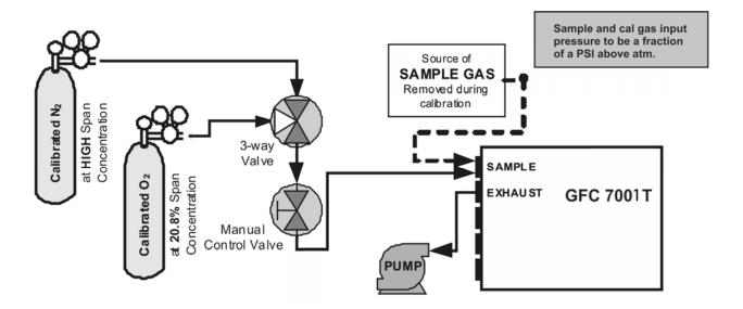
Figure 9-7: O<sub>2</sub> Sensor Calibration Set Up
